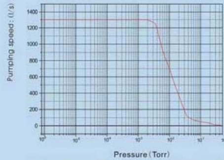
FF-200/1300E compound molecular pump (1300 l/sec)
